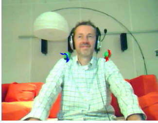
Fig. 6. Two green spheres placed on the user's shoulders are tracked in realtime (red and blue trajectories)
